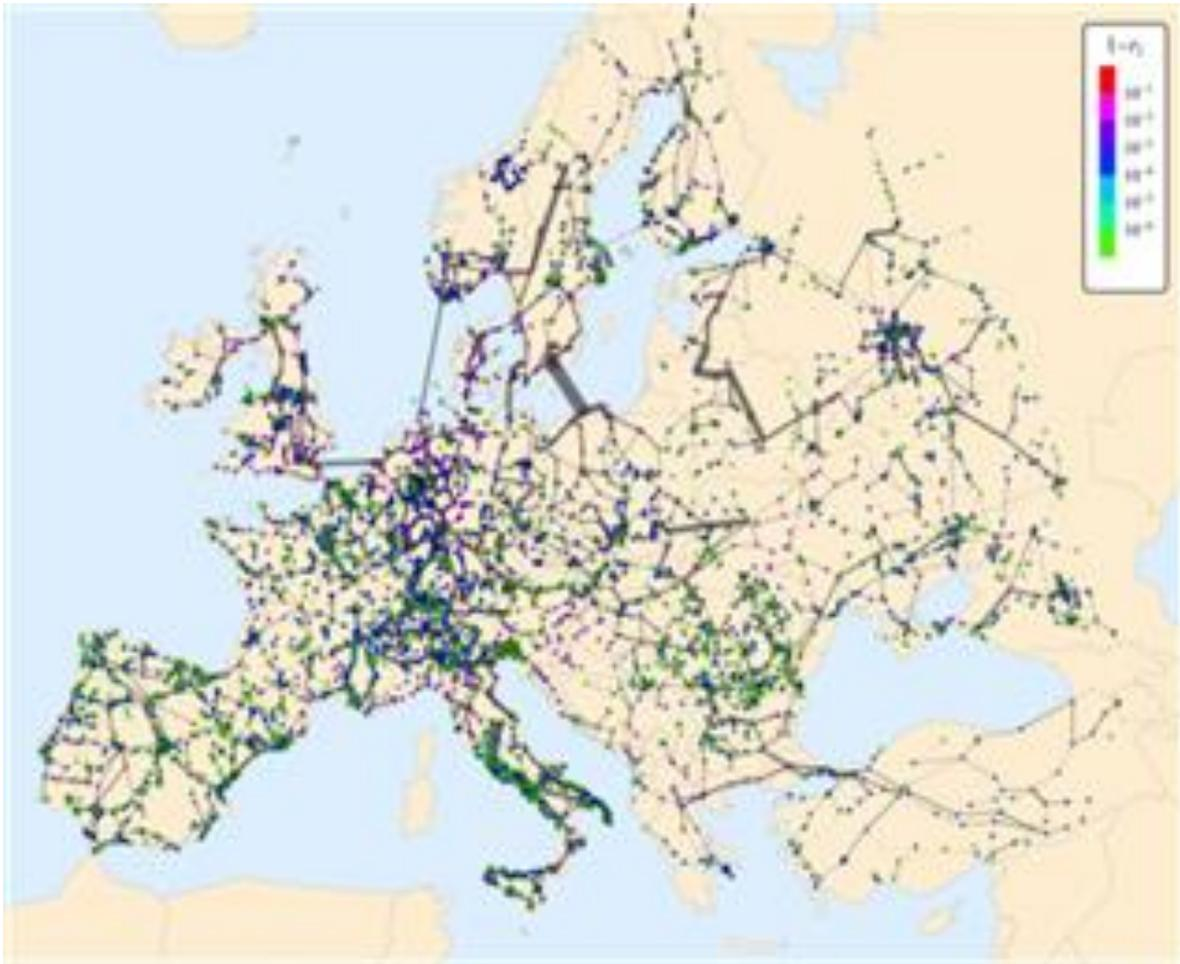
**Figure 7.8.** Local Kuramoto results encoded by the color map as  $1-r_i$ . Red corresponds low local synchronization, green to high synchronization. The width of gray edges is proportional to the amplitude of the power flow.
